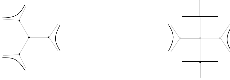
FIGURE 1. Left, a reduction on a 3-vertex with 3 3-neighbors, followed by II-reductions on those neighbors, destroys 6 edges and 4 3-vertices. (The original graph’s edges are shown in grey and the reduced graph’s edges in black.) Note that Algorithm A does not actually force any particular II-reductions after a III-reduction, but Algorithm B will do so. Right, a reduction on a 4-vertex with k 3-neighbors ( k = 2 here) destroys 4 + k edges and 2k - 4 3-vertices ( k 3-vertices are destroyed, but 4 - k 4-vertices become 3-vertices). The algorithm and analysis make no assumptions on the local structure of the graph; the figure is merely illustrative.
